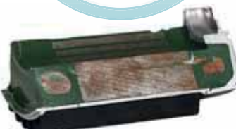
Insulated motor winding cross section
